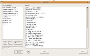
With NrpTerm it is possible to send one or more commands to an NRP-Z series Power sensor very user-friendly and see all the data sent by the sensor in a well arranged display. To start the program simply go into the NrpTerm directory and enter the program name ./NrpTerm - Before you do so,
